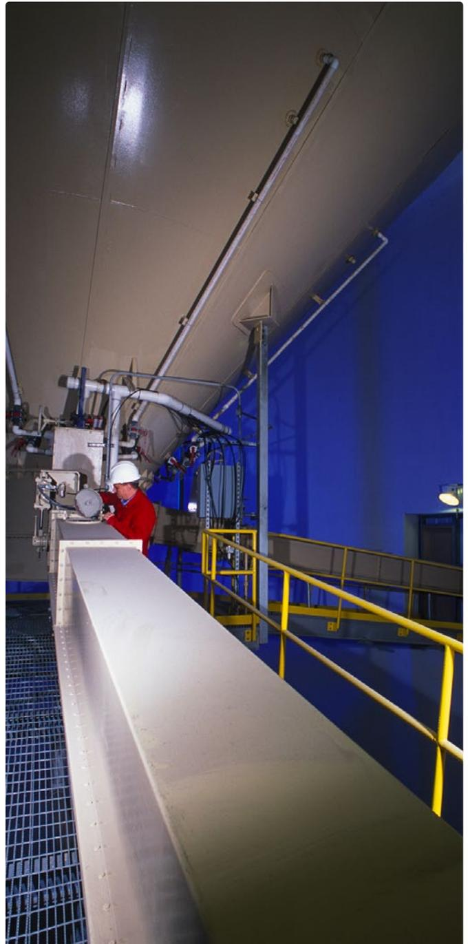
Airslide® gravity conveyor
